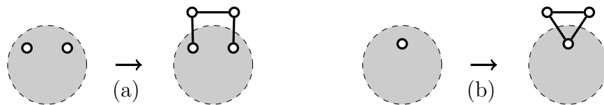
Figure 10: For any starting graph satisfying the count e = \frac{3}{2}(v - 1) , we can add two vertices and three edges to retain the isostatic count, bridging any pair of vertices of the original graph (a). Alternatively, we can ‘add a triangle’ to the original graph, which in the expanded graph, is equivalent to adding a six-ring (b).
